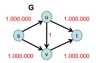
If we always pick an augmenting path along the edge of capacity 1, it takes 2.000.000 (!) augmentations to reach a maximum flow.
