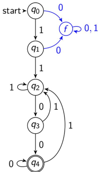
$$\begin{aligned}\delta(q_0, 100) &= \delta(\delta(q_0, 10), 0) \\ &= \delta(\delta(\delta(q_0, 1), 0), 0) \\ &= \delta(\delta(q_1, 0), 0) \\ &= \delta(f, 0) \\ &= f\end{aligned}$$
