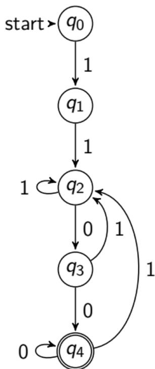
$$\begin{aligned}\delta(q_0, 11100) &= \delta(\delta(q_0, 1110), 0) \\ &= \delta(\delta(\delta(q_0, 111), 0), 0) \\ &= \delta(\delta(\delta(\delta(q_0, 11), 1), 0), 0) \\ &= \delta(\delta(\delta(\delta(\delta(q_0, 1), 1), 1), 0), 0), 0) \\ &= \delta(\delta(\delta(\delta(q_1, 1), 1), 0), 0) \\ &= \delta(\delta(\delta(q_2, 1), 0), 0) \\ &= \delta(\delta(q_2, 0), 0) \\ &= \delta(q_3, 0) \\ &= q_4 \in F\end{aligned}$$
